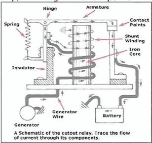
An obvious failure mode is the contact points. As they open and close, a slight spark is generated, eventually eroding the material on the points until they either "weld" themselves together or become so high in resistance that they won't conduct current when closed. In the first case the battery would discharge through the generator overnight and in the second there would be no charging to the system.
